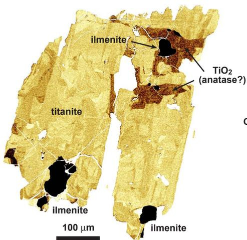
False-color back-scattered electron (BSE) image of relict(?) magmatic ilmenite replaced by hydrothermal titanite+anatase(?), from actinolite-albite-titanite veins cutting Na-Ca metasomatized diorite, Duff Creek, Cortez Mountain metasomatic iron-oxide-Cu-Au (IOCG) district, NV.
